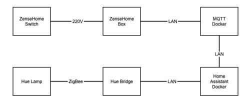
Pressing the Switch send a signal over 220V cable to the ZenseHome box, that post a message on a MQTT Tpoic, that Home Assistent picks up, and sends a toogle to the Hue Brige, that informs the Lamp over ZigBee..
