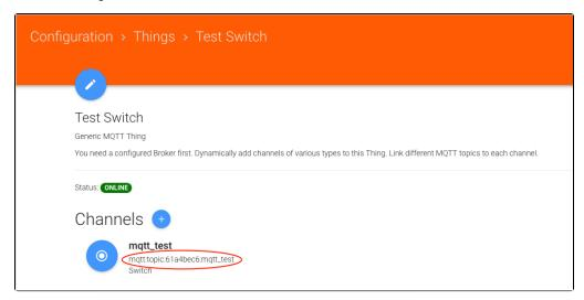
The Thing is the "physical" device, like a light Switch, and the Channel(s) is the properties the Light switch has - now, a switch has only On/Off, but other Things may have several properties, an engine can have On/Off, Temperature, Rounds Per Minute etc.
