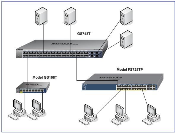
Figure 8. Backbone Switching
