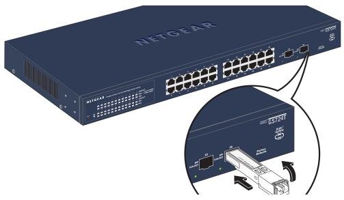
Figure 11. Install an SFP Gigabit Ethernet Module
